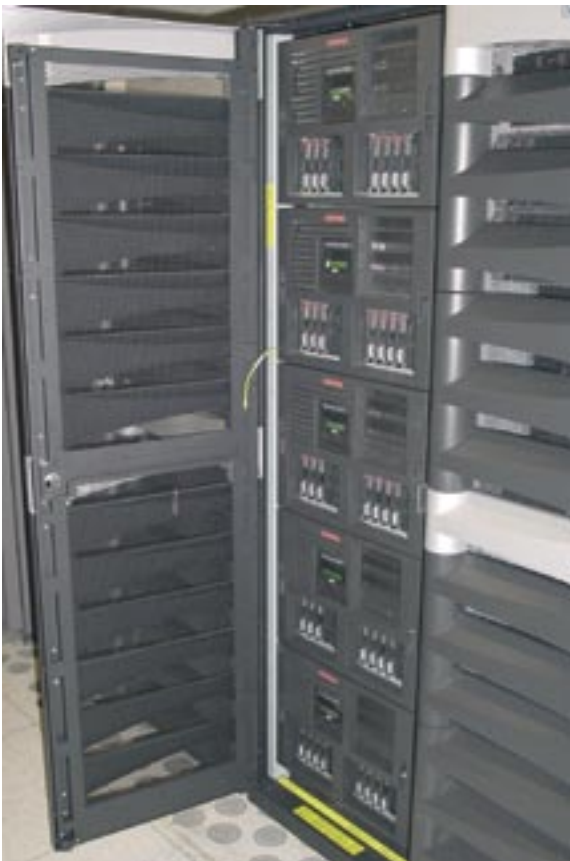
ATHOS (HP SC45 Cluster, Alpha-CPU und Quadrics Switch Technology)
