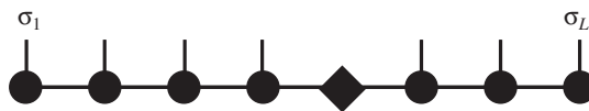
Fig. 8. Graphical representation of an exact MPS obtained by a sequence of singular value decompositions, starting from the left and right. The diamond represents the diagonal singular value matrix. Matrices to the left are left-normalized, to the right are right-normalized.
