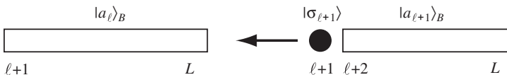
Fig. 12. A block B of length L - \ell - 1 is grown towards the left to a block B of length L - \ell by adding site \ell + 1 .
