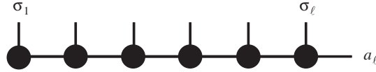
Fig. 11. Graphical representation of the recursive construction of a state |a_\ell\rangle by contraction (multiplication) of A -matrices. Contractions run over all connected legs.
