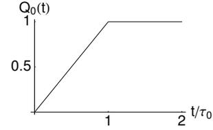
Figure 2: Time dependence of primary charge.
